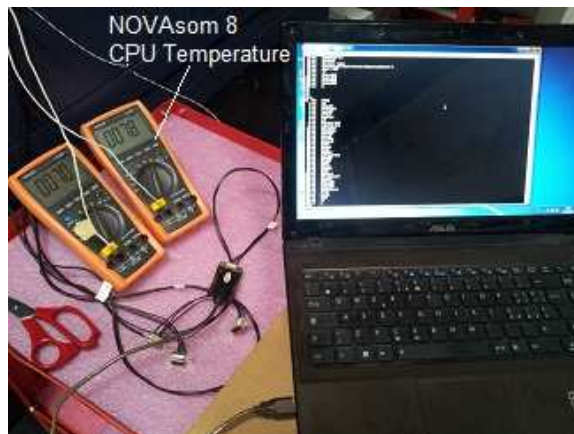
Figure 10: Temperature measured on NOVAAsom 8 processor after 2 Hours at +70°
