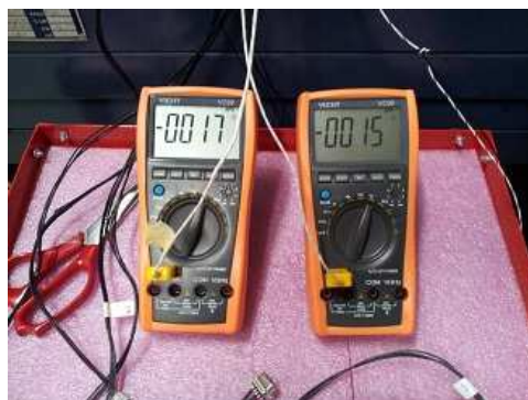
Figure 5: Temperature measured on NOVASom 8 case processor after power on at -20° (Multimeter on right side)
